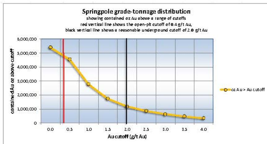
**Figure 2: Contained Au distribution by cutoff**
