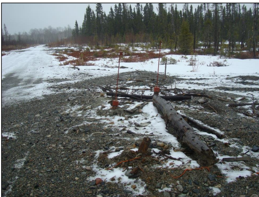
Figure 12.5 View of the Cased Drill Collars with the Metal Rods Denoting Hole Number
